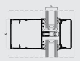
CW 60 is an excellent thermally improved curtain wall system for large glass surfaces (cassettes can hold a weight up to 450 kg per glass panel), sloping and vertical or curved constructions, especially for renovation projects.
