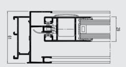
The CP 45Pa is a non-insulated sliding system that has been designed to respond to new aesthetical demands. The system is available in functional and softline design. The profile width is reduced to a minimum allowing a maximum of light into the building.
